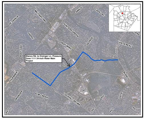
✓ The project will require open cut and bore construction methods that reach depths up to 18 feet. Bore construction will take place at the intersection of George Rd. and Lockhill-Selma, at the intersection of Fairfield Bend & the drainage channel, in the drainage channel behind Gable Village Dr, and as well as the intersection of George Rd. and NW Military. The contractor will need to excavate through rock in various areas within the project.
